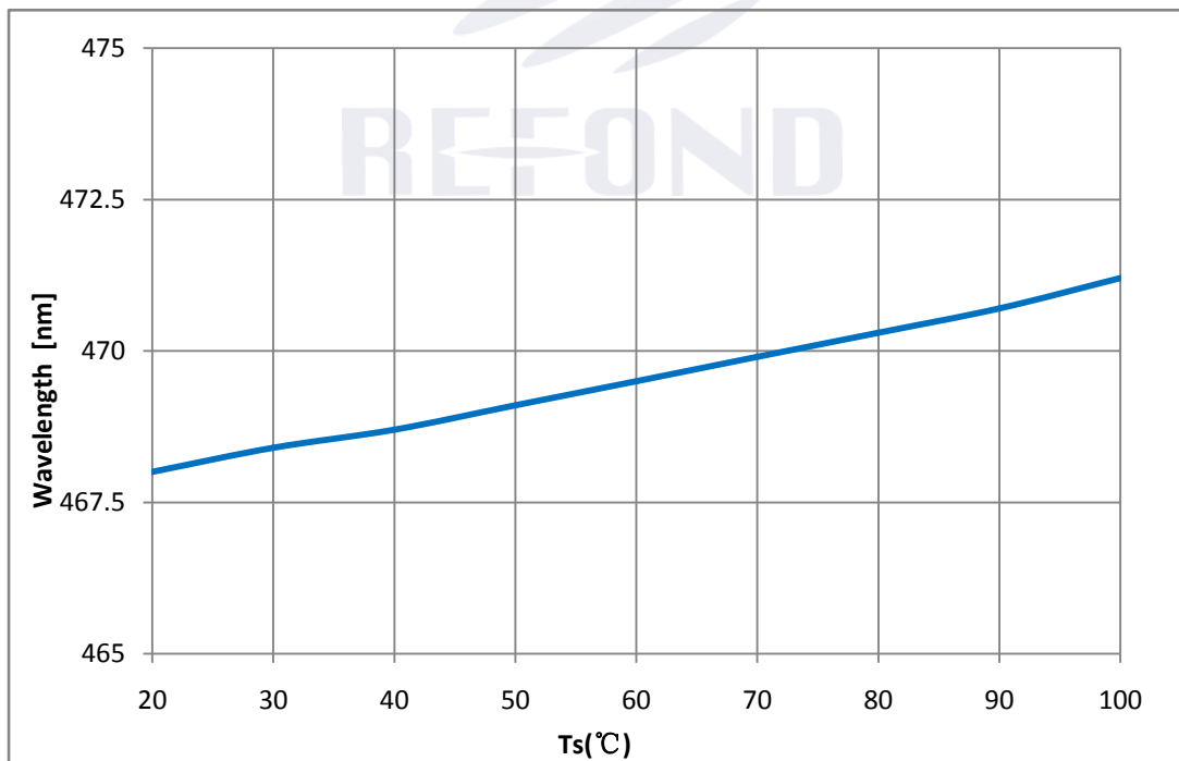
Fig 1-12 Wavelength Vs. Pin Temperature 波长与引脚温度特性曲线
